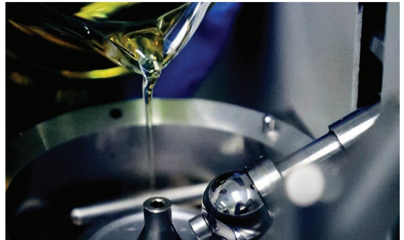
Figure 2: Mini Traction Machine
