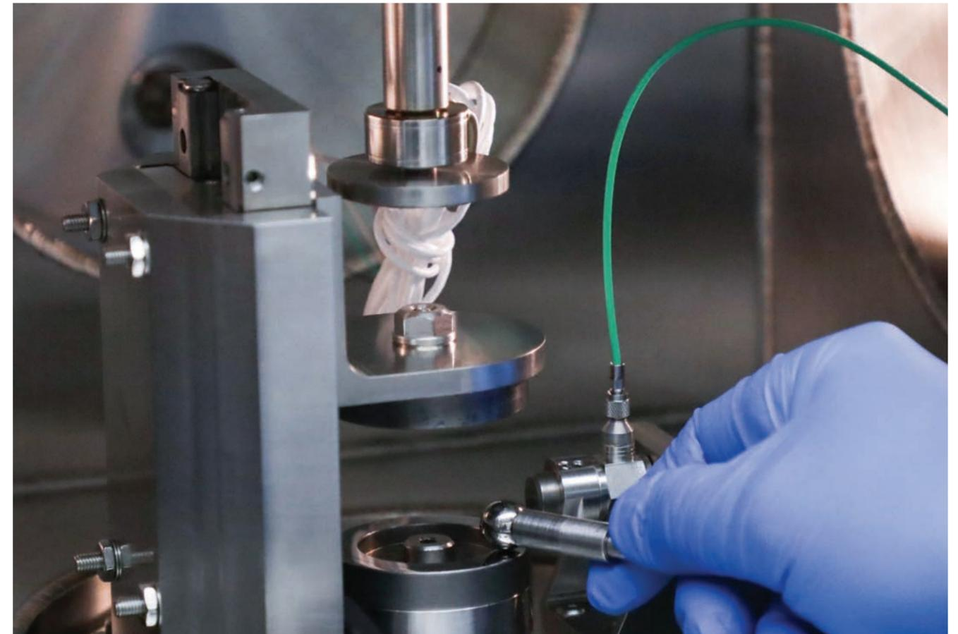
Figure 1: Spiral Orbit Tribometer
