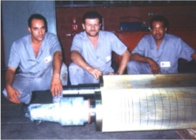
(Left) Denilson Stanguine Ferreira, Irlei Felipe, and Paulo Sergio Magalhães de Souza, three members of the Ibéria maintenance department, pause after installing FARO shielded corrugator roll bearings lubricated with NyeCorr 140 PFPE/PTFE grease. The FARO/Nye system significantly reduces the cost of converting singlefacers lubrication from oil to high-temperature grease.
