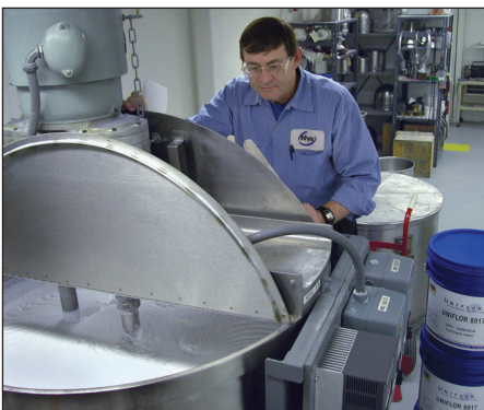
Nye Technician mixes a 1,500-lb batch of UniFlor™ 8917 at the company's Fairhaven, Massachusetts, headquarters.
