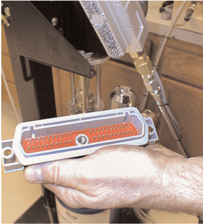
Figure 3: Dispensing the Grease This semi-automatic connector grease dispensing system, custom designed by LCC/Dispensit of Indianapolis, Ind., allows the operator to dispense minute amounts of grease in multiple locations simultaneously, quickly, and precisely.
