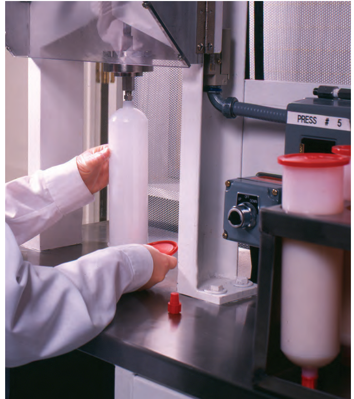
Clean room, clean grease. Clean air for a 10-foot mini-environment blankets the working surface, where lubricants are ultrafiltered and packaged in a Class 100 environment.
