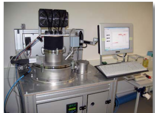
Picture: Nye's ASTM E-595 Outgassing Test Rig
