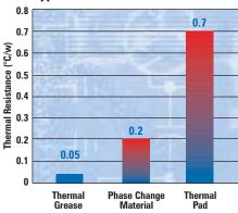
Compared to thermal pads and phase change materials, thermal grease offers the lowest possible thermal resistance.
