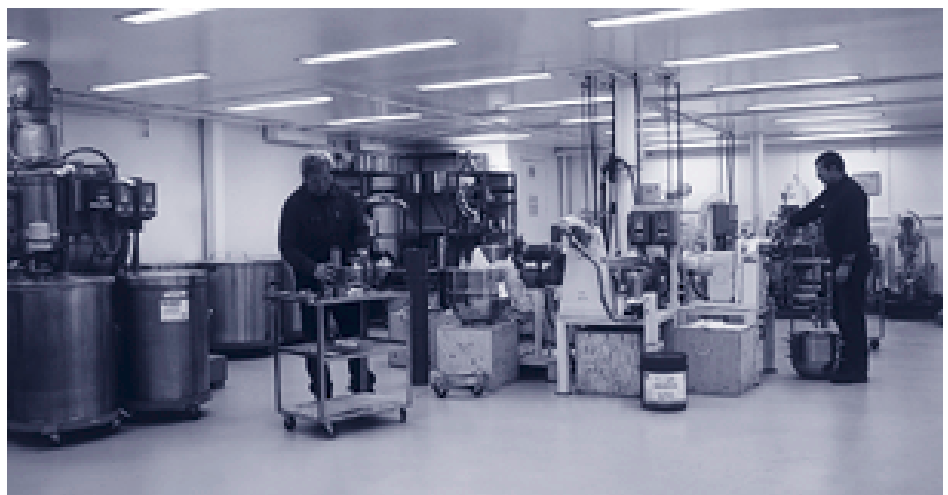
On a cellular level. A three-person team, using dedicated equipment, produces all of Nye's PFPE oils and greases in the new UniFlor Cell.
