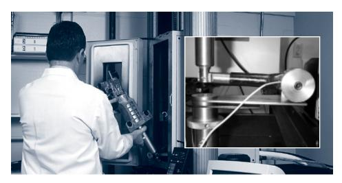
Nye has used the Instron 5566 to pre-qualify lubricants for master cyclinders, steering columns...and now for ball joints (inset). The Instron performs tensile, compression, shear, peel, tear, flexural, and other tests on a wide variety of materials and components.
