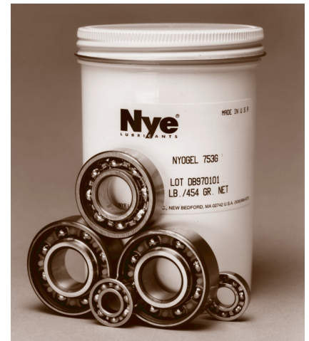
NyoGel 753G, an electrically conductive bearing grease, helps extend bearing life by allowing static discharge to pass through the bearing instead of pitting the rolling element or fluting the raceway.
