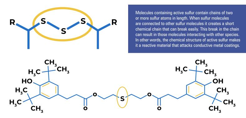
In inactive sulfur compounds, molecules contain fewer than two sulfur atoms in length. In the example shown above, sulfur is connected to carbon or oxygen, which creates a tight chemical structure. Because the structure is so tight, the sulfur molecules do not break off the chain. Thus, they cannot react with the conductive metal coating on the connector surface to create tarnish.
