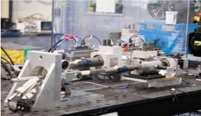
Nye's Application Engineers will work with you to design and build custom test equipment that validates our lubricant for your application. With our custom modification and a collaborative partnership, we can ensure that the test rig meets your application requirements. Nye engineers are currently using the data collected by our test rigs to formulate next-generation greases for the Automotive Industry.
