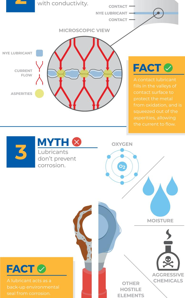
Lubricants seal contact metals from oxygen, moisture, aggressive chemicals and other hostile elements.
